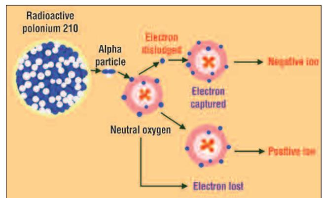
**Figure 2. In alpha ionization, polonium 10 collides with air molecules and knocks out electrons.**
