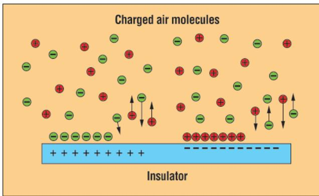
**Figure 1. Neutralizing a surface through bipolar air ionization.**
